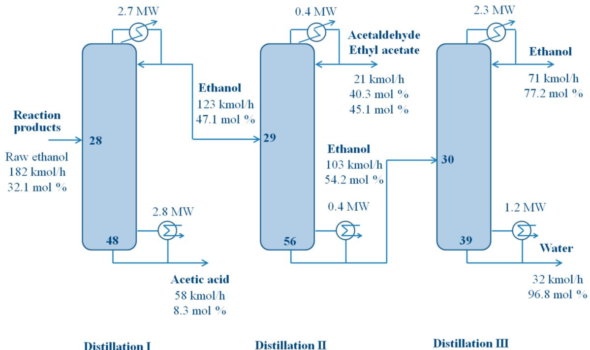
**Figure.** Schematic diagram of distillation columns in the conventional process for the ethanol concentration. The numbers in the columns indicate tray numbers, counted from the top.
