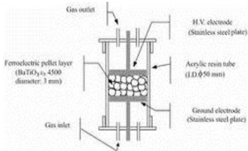
Figure 1: Schematic diagram of the packed-bed reactor.
