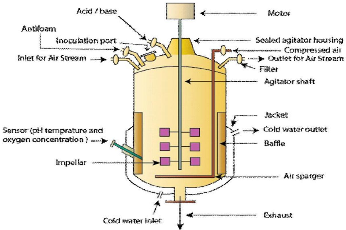
Continuous stirred-tank reactors (Fermenter: Equipment design) (Source: nptel@iitm.ac.in) CSTRs consist of a tank, usually of constant volume, and a stirring system to mix reactants together. Also, feed and exit pipes are present to introduce reactants and remove products.
