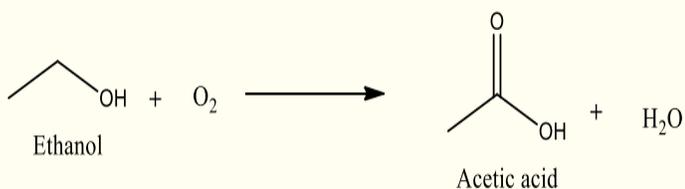
Scheme 4 Production of acetic acid by fermentative oxidation of alcohol
