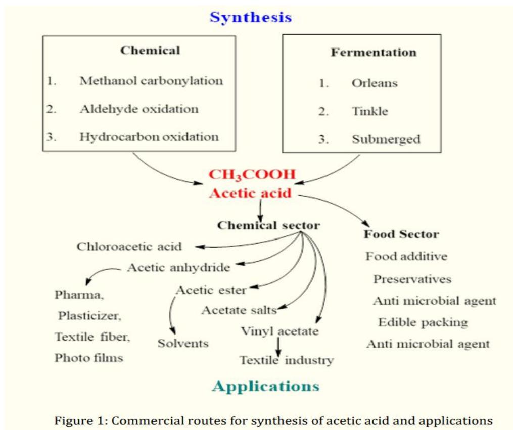
Figure 1: Commercial routes for synthesis of acetic acid and applications
