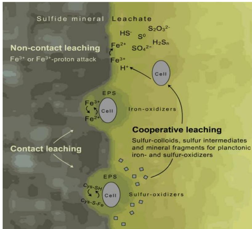
Figure: **Sulfide mineral bacterial leaching:** Bacterial cells oxidizing the ferrous iron back to ferric iron while using slightly different contact mechanisms with the metal.
