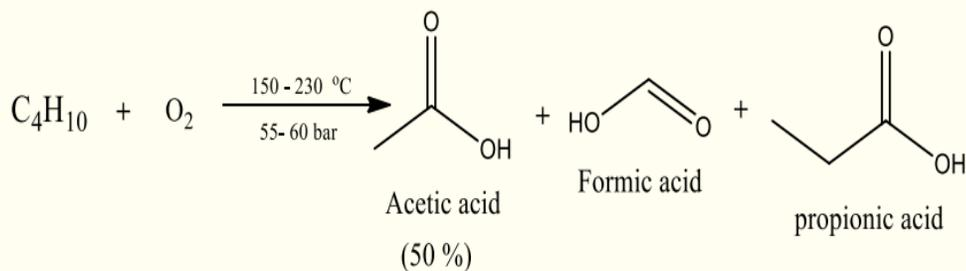
Scheme 3 Production of acetic acid by hydrocarbon oxidation
