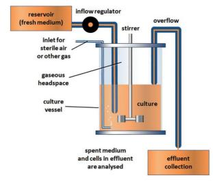
**Figure 8** Continuous culture system, 'chemostat'. The main vessel contains a well-stirred culture medium, which is replenished from the reservoir. The culture vessel maintains a constant volume of culture, since the inflow of a fresh medium from the reservoir equals the outflow of spent medium (overflow) from the vessel.
