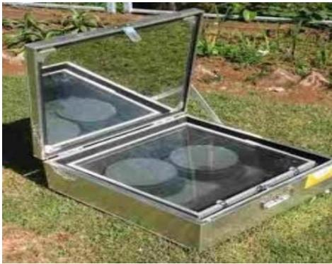
Fig 3- Box Type Solar Collector
